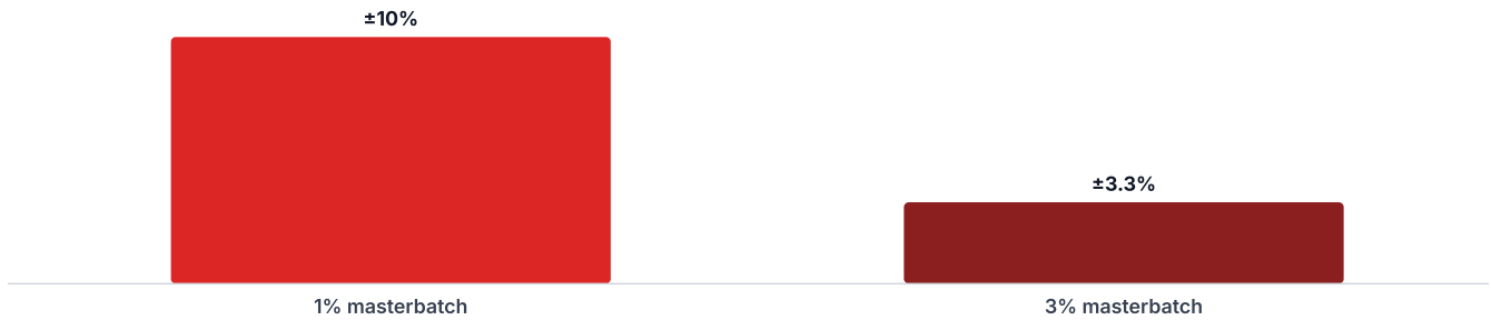
Figure 8 Relative deviation of a \pm 0.1 g dosing error by masterbatch ratio
